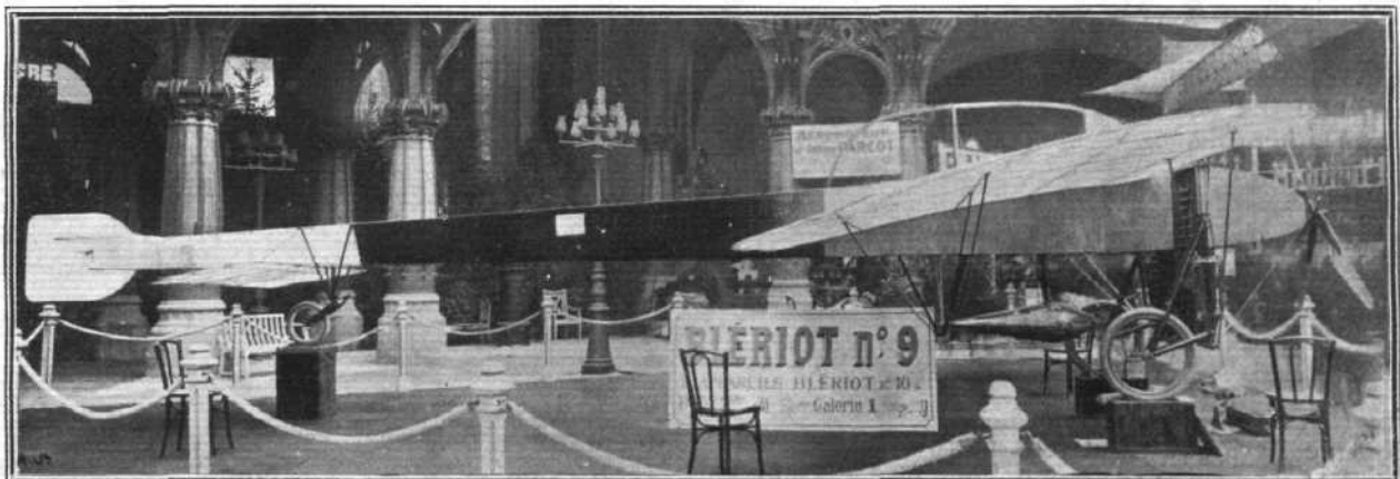
PARIS AERO SALON.—Side view of the Blériot Monoplane “No. 9.” The central part of the body, which is black, is the flexible radiator.
