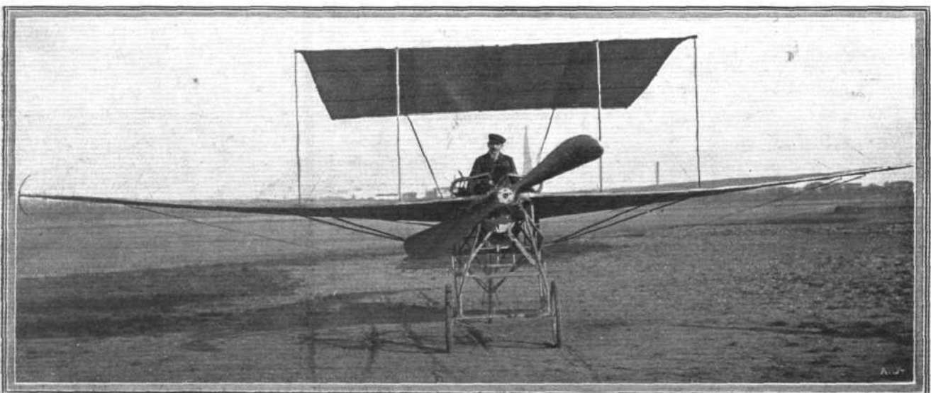
THE OBRE BIPLANE.—Front view of the Obre aeroplane, which came to grief in its early trials, as recorded last week. Although essentially of the biplane type, this machine has a very small expanse of upper deck. It has a light monoplane tail and rudder behind, which are invisible in the above view. The span of the lower deck is 10 metres; the engine is a 50-h.p. 3-cyl. Anzani.
