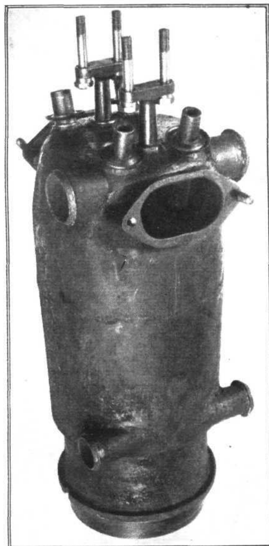
Fig. 6.—The Mercedes cylinder.
