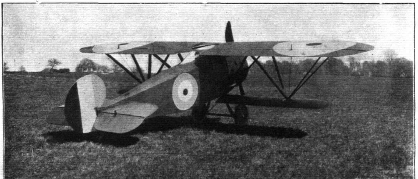
THE AVRO "SPIDER." —Note the unusual strutting arrangement.
