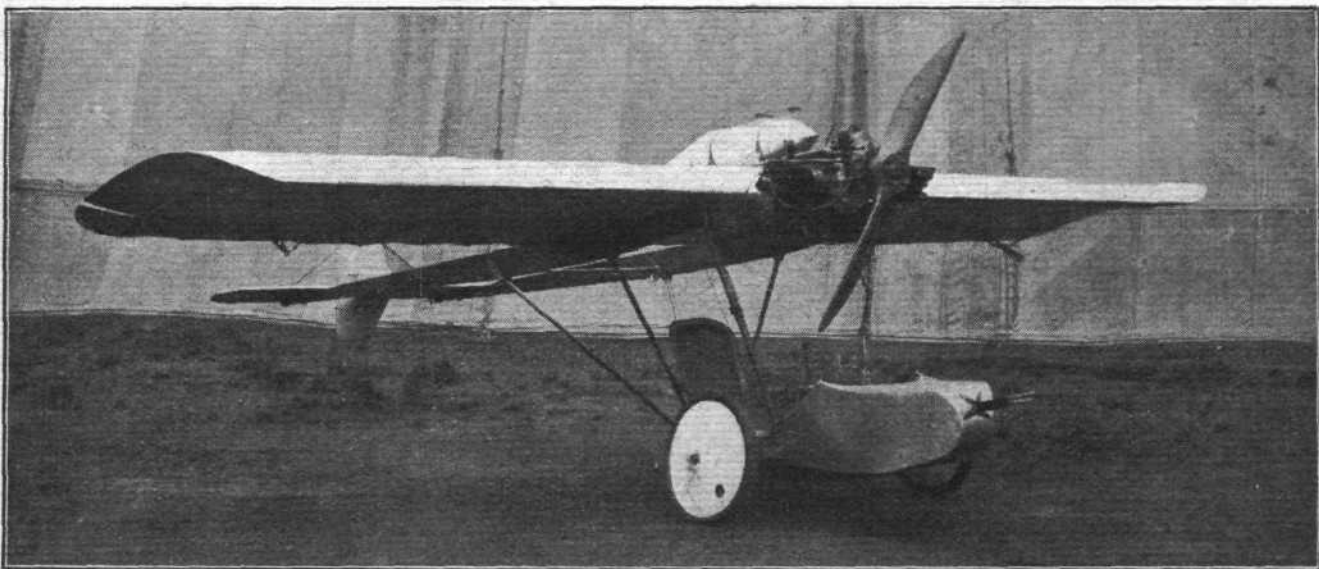
The B.A.T. "Crow" (F.K. 28), the "motor-cycle of the air." It has a span of only 15 ft., and is fitted with [a 40 h.p. "A.B.C. Gnat"]
