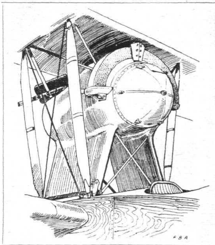
The engine mounting on the F.B.A.
