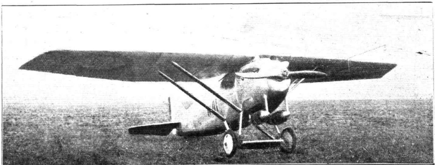
THE DEWOITINE MONOPLANE, 300 H.P. HISPANO-SUIZA ENGINE : The machine actually exhibited at Prague is fitted with the new type Lamblin radiators mounted on the struts of the undercarriage.
