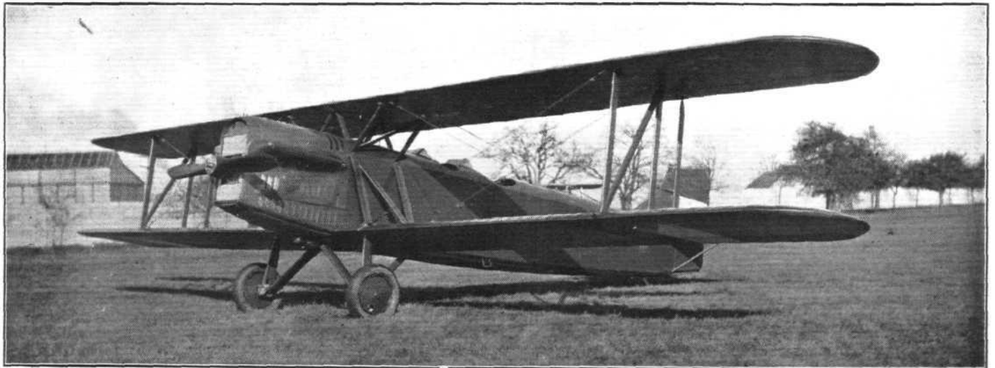
AN ALL-METAL CZECHOSLOVAK MACHINE : The Vojenska-Smolik S.16 is a long-distance reconnaissance two-seater or day bomber. Three-quarter front view.
