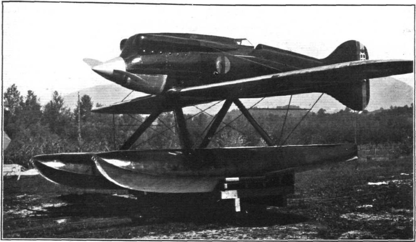
THE ITALIAN DEFENDERS : Three-quarter front view of the Macchi M.52. The wings are slightly swept back. The floats are of wood construction.
