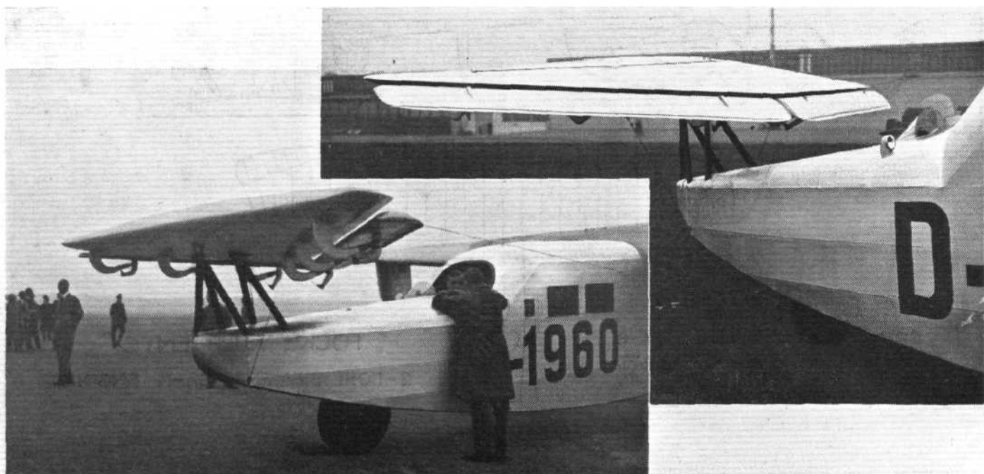
THE FOCKE-WULF "ENTE" : Two views of the front plane. Note the slot arrangement of the elevator flaps.
