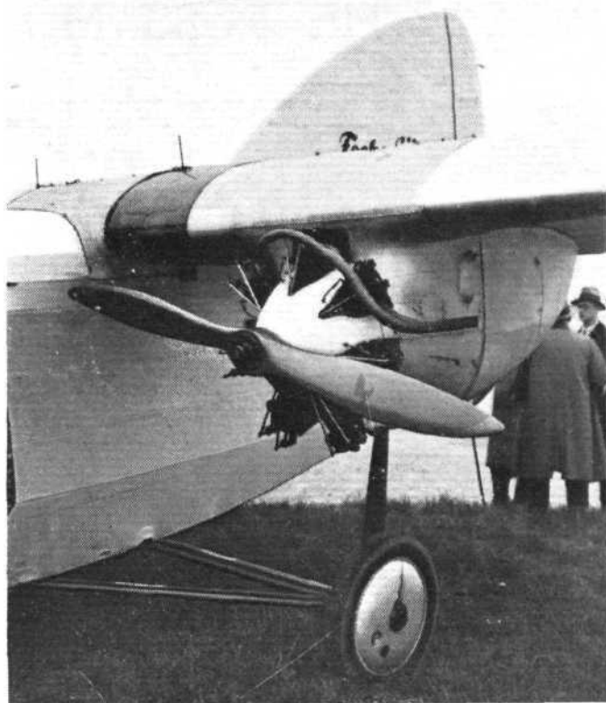
One of the Power Plants of the "Ente": These are Siemens Sh-14 type, of 110 h.p. each. The under-carriage consists of a horizontal Vee and a telescopic strut to the engine mounting.
