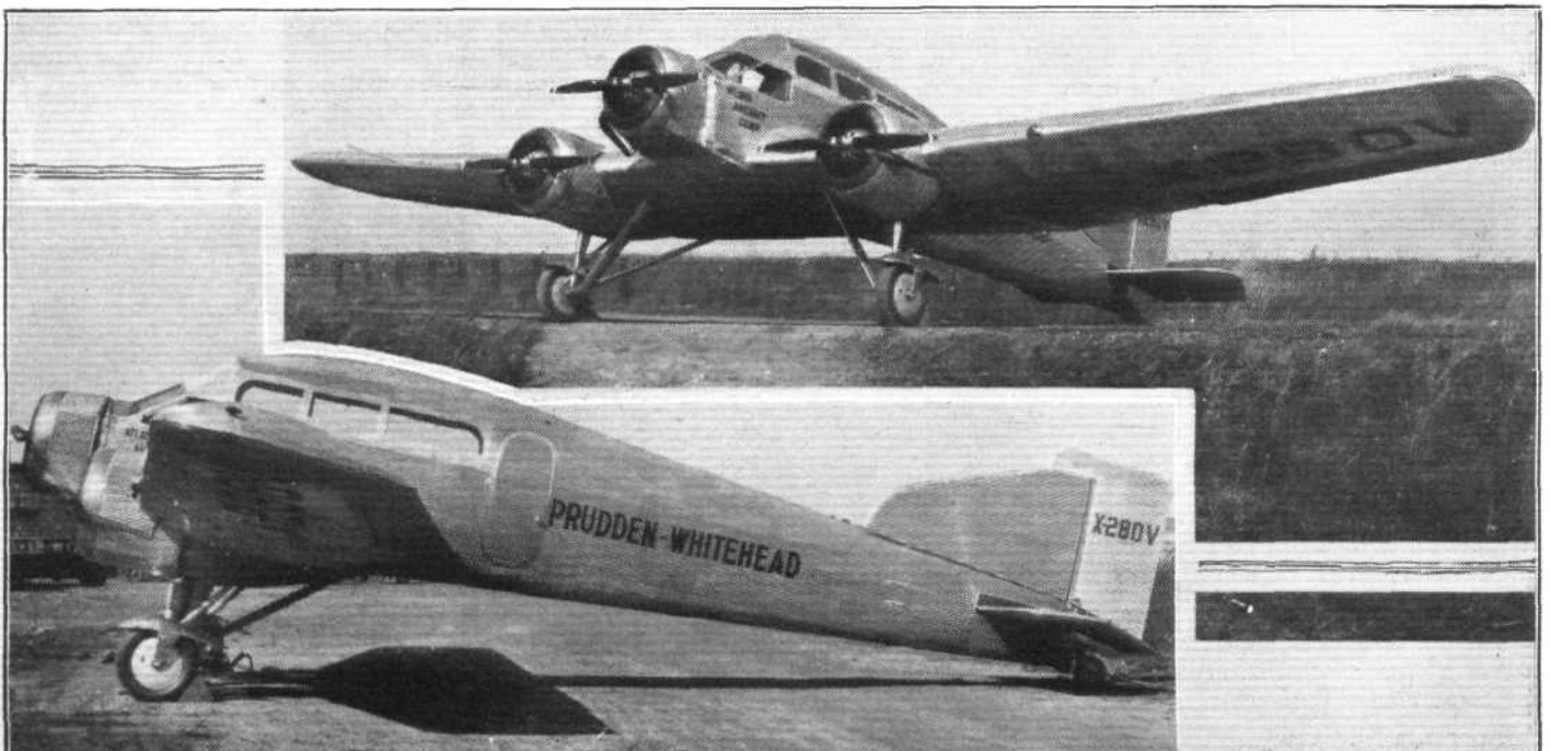
AN AMERICAN ALL-METAL COMMERCIAL MONOPLANE: The Prudden-Whitehead low-wing monoplane, powered with three 240-h.p. Wright J6-R760 engines, and carrying eight passengers.
