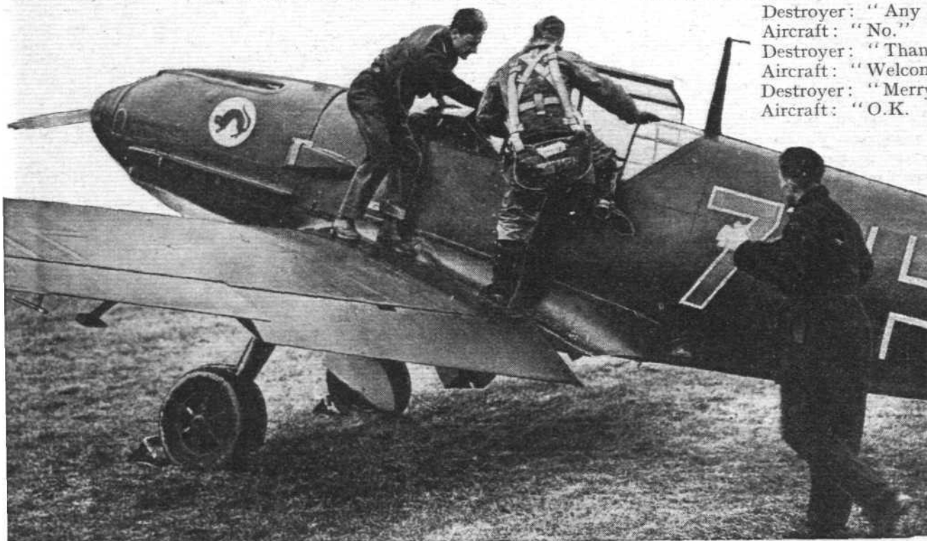
A German fighter pilot enters his Me 109. It will be seen that this is one of the later machines with Daimler Benz engine. The splayed-out undercarriage and the slotted flaps are points worth noting.
