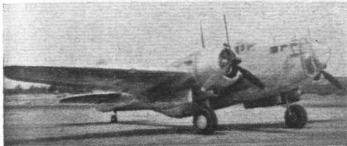
THE BALTIMORE (187) : It resembles the Maryland but has a deeper-sectioned fuselage which drops down at the upper gun-turret amidships. The trailing-edges of its wings are "webbed" to the ends of its long engine-nacelles.
