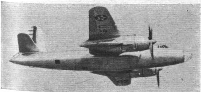
THE MARAUDER (B-26) : A larger machine than the other two Martins, it is beautifully streamlined and has a neatly faired gun position in its tail. Note the mounting of the wings almost amidships and the long nacelles.
