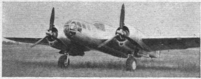
THE MARYLAND (167W) : Doing wonderful service with the R.A.F. in the Middle East ; it can be identified by the comparatively small section of the rounded nose and the step-up in front of the tailplane as shown on the drawing below.
