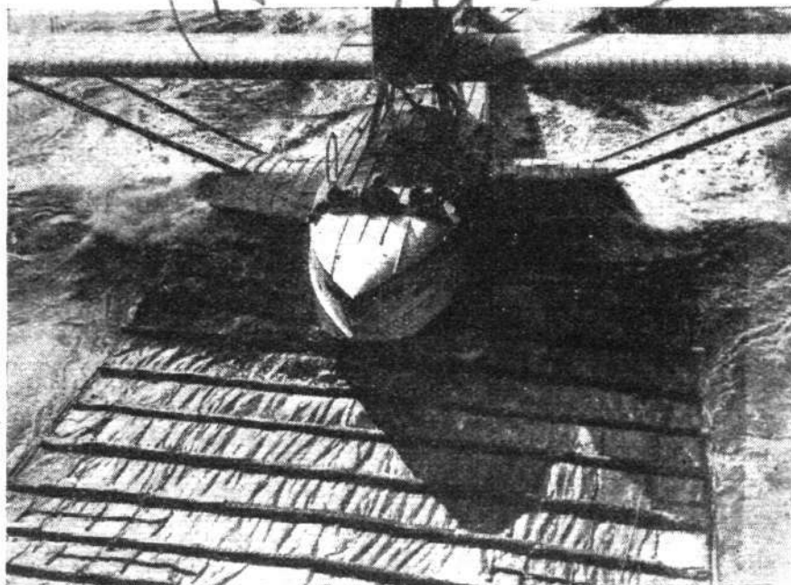
A Dornier Wal flying boat on the landing apron of the mother ship Westfalen . The machines were catapulted off the deck.
