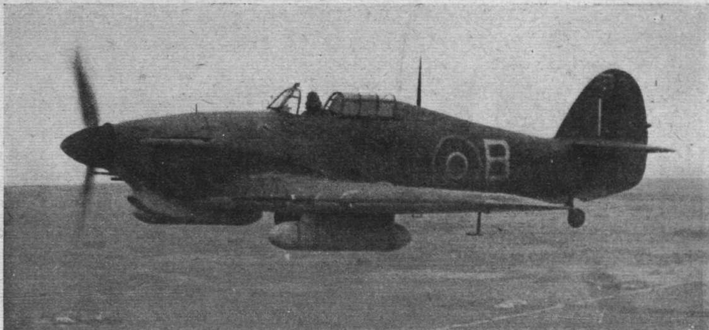
RANGE AND POWER : A four-cannon Hurricane IIC over Tunisia. The long-range tanks enable escorting fighters to cover the bombers during the whole journey.
