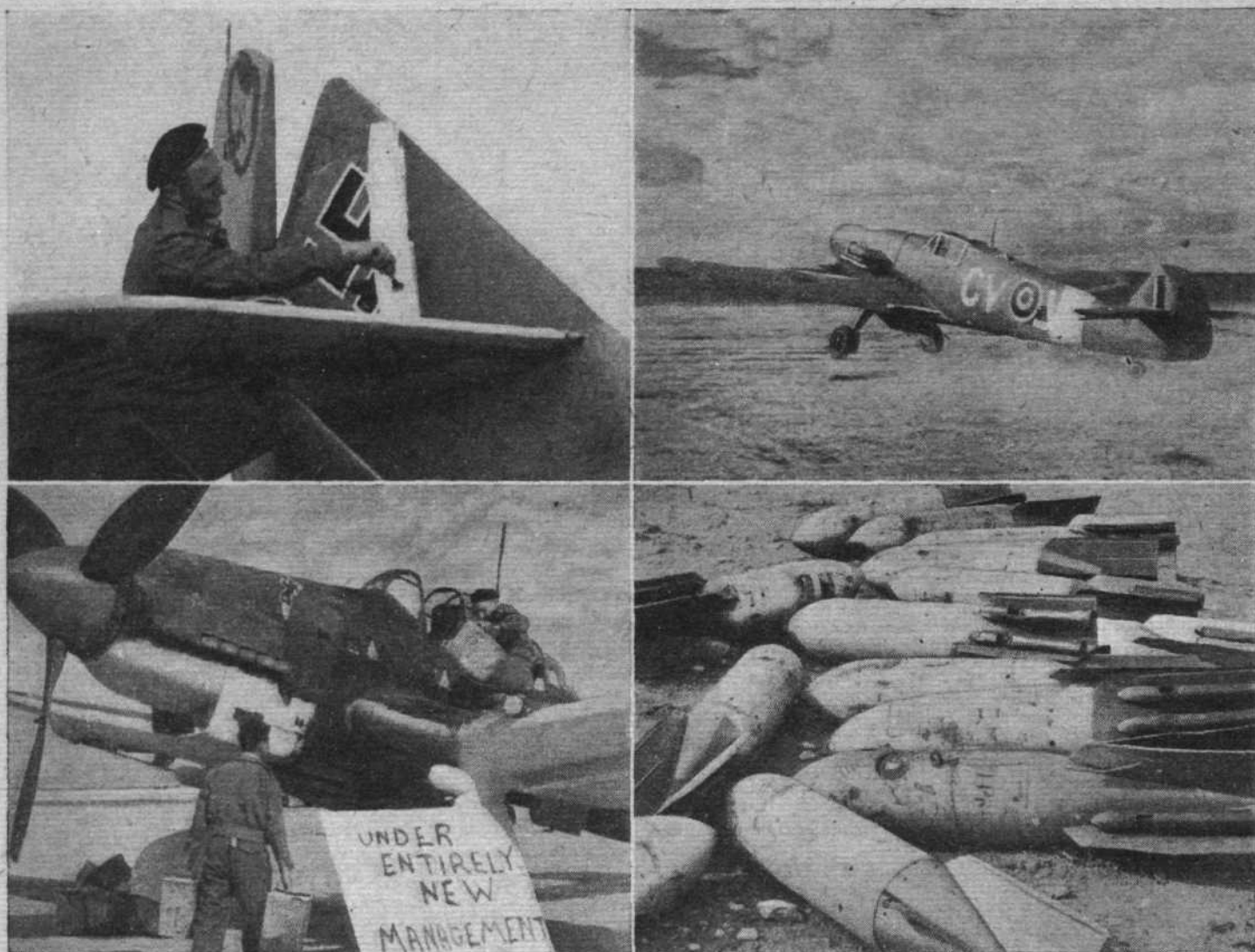
TRYING THEM OUT: A number of enemy aircraft captured in Libya have been made serviceable and given R.A.F. markings. (Top left) With much satisfaction the swastika is blotted out on the tail of a Me 109E. (Top right) An adapted Me 109F taxis in after a test flight. The split flaps are seen opened out to act as an air brake. Acute tail buffeting would be expected from the operation of these flaps and this may have some bearing on the high tailplane position. (Bottom left) Filling up the fuel tanks of a Junkers Ju 87D. (Bottom right) A number of "whistlers," the music of which will be appreciated by the Germans.
