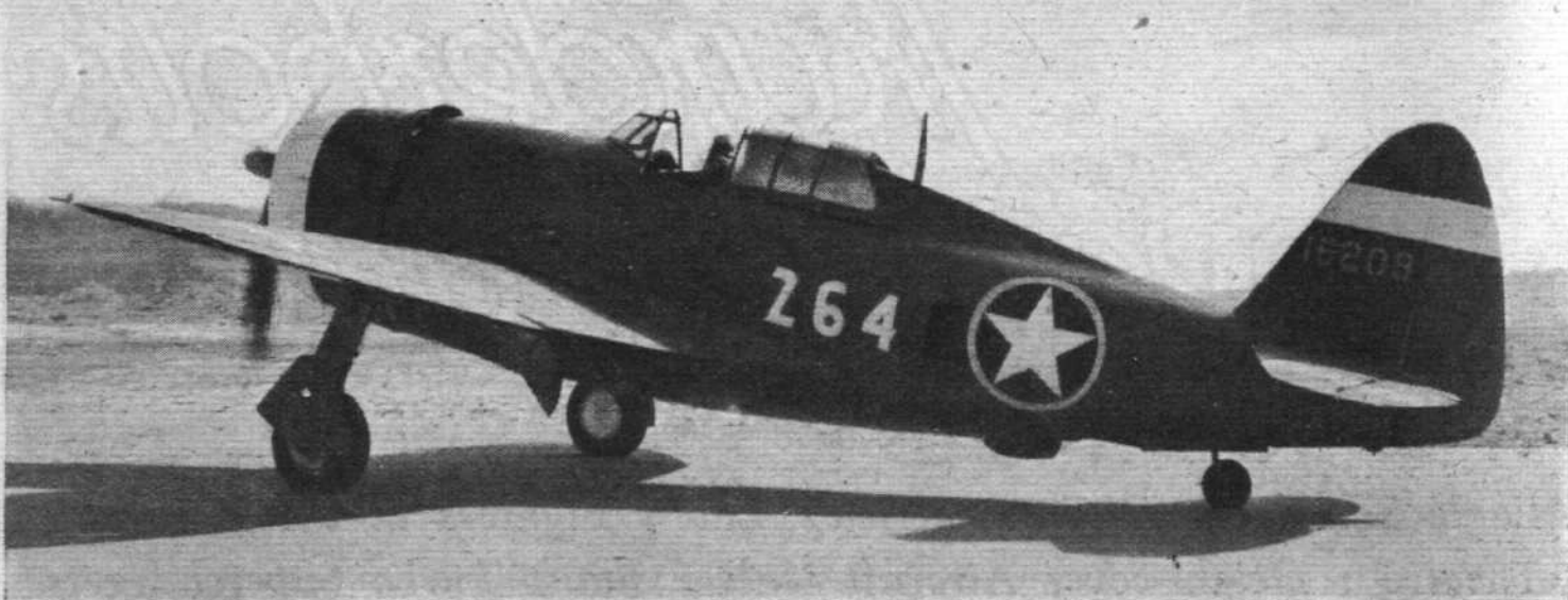
Two general views of the P.47. The four-bladed airscrew of 12-ft. diameter gives a reasonable ground clearance with short undercarriage legs. The cockpit cover slides straight back. "Flight" photographs.
