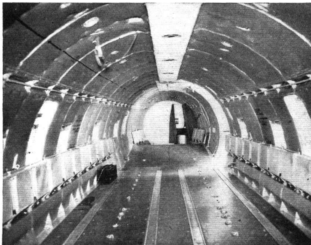
INSIDE A COMMANDO : The walls are lined with Fiberglass "blankets" made of very thin glass threads set in a synthetic resin \frac{1}{2} in. thick. The weight of the material is only 1 oz. per sq. ft.
