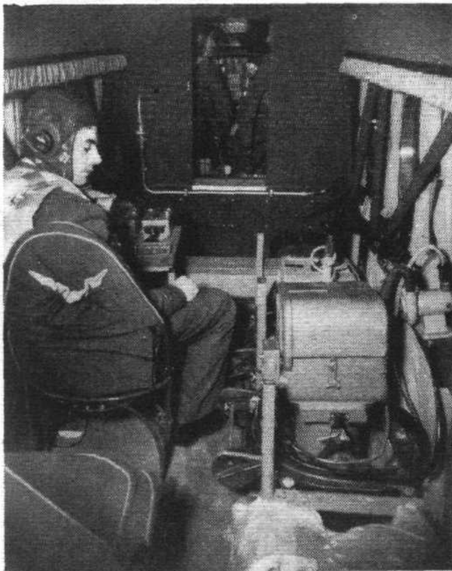
PEACETIME P.R.: (Above) The interior of one of the R.A.F. photographic Ansons recently engaged in mapping 50 sq. miles of Central and West London. In the camera repair section at upper right adjustments are being made to an F.52 20" lens. The need for speedy printing, developing and drying of film is met by the multi-printer (right).
