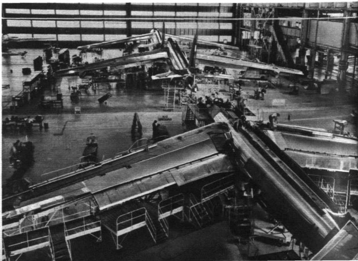
“Remachable” transonics: Boeing B-47A medium-range Stratojets are now coming off the production line at Wichita, first of a batch of 75. The B-47 is an ingenious structural interpretation of the Mach theme in its application to the thin, flexible, swept-back wing.
