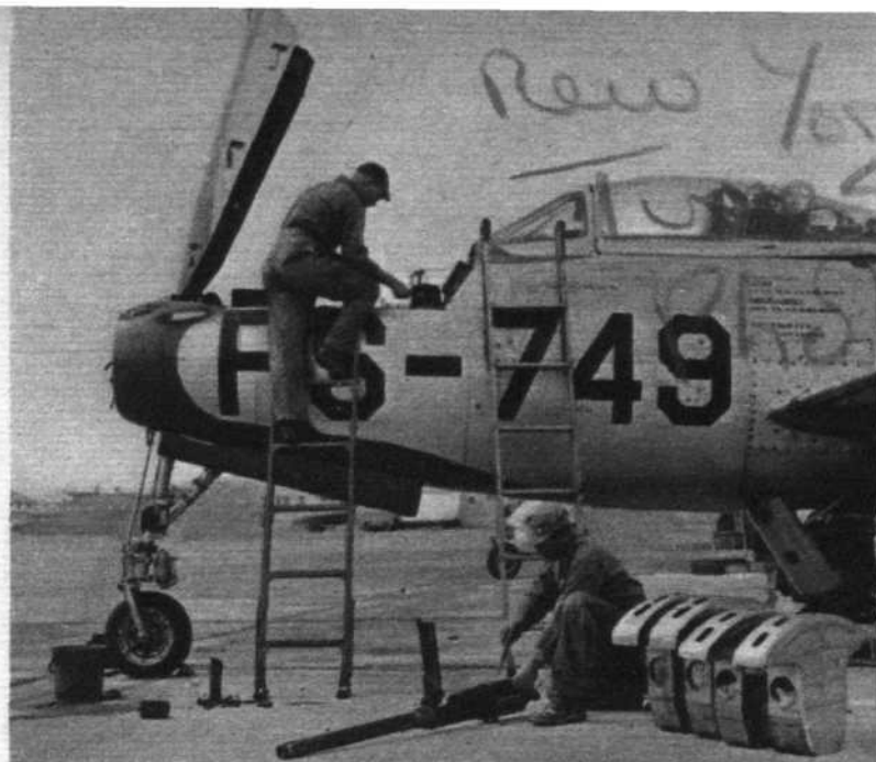
"It is futile to derive comfort from the American worship of the 0.5 in calibre . . ." Armourers at work on a Republic Thunderjet, mounting six Colt (Browning) -type guns of half-inch calibre
