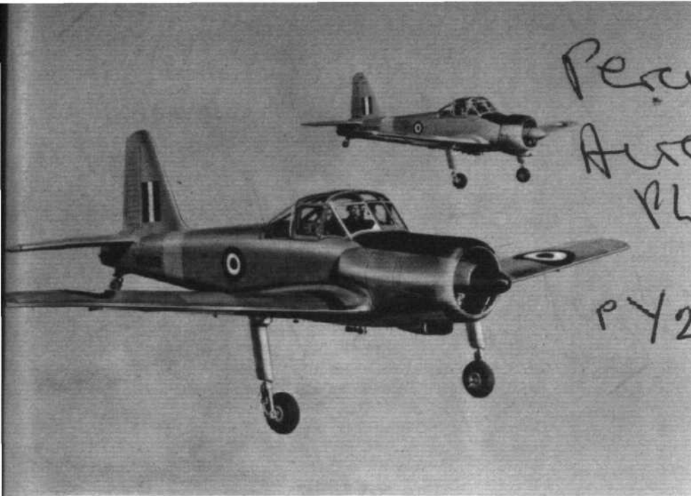
The two types of Percival P. 56 basic trainer: The external differences between the Cheetah-powered Mk 1 and the Leonides-powered Mk 2 (in foreground) lie chiefly in the cowling lines.
