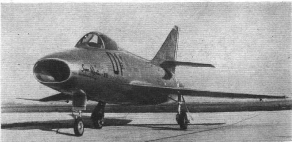
In common with the North American Super Sabre, France's Marcel Dassault Super Mystère (otherwise known as Mystère IVB1) has a "flattened" intake.
