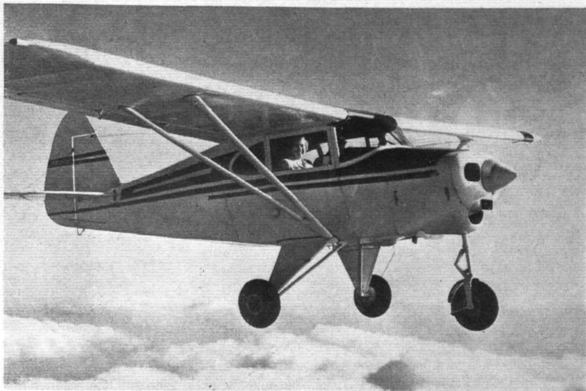
The Piper Tri-Pacer 150 illustrated here is practically identical with the machine described in this article; it is, in fact, the latest 1955 version with slightly larger airscrew and a 150 h.p. version of the Lycoming engine. The version described has a 135 h.p. engine. Upholstery colours offered to customers are "Tennessee red, Miami blue or forest green."
