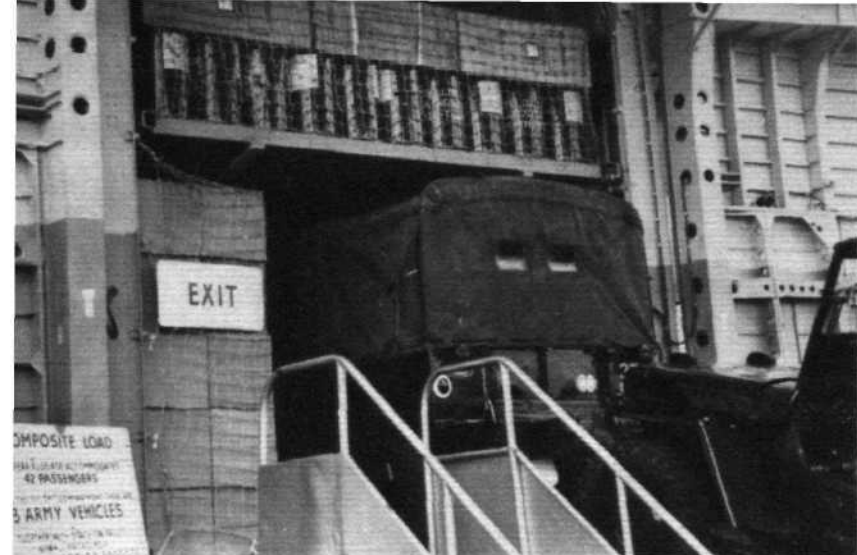
The Blackburn Beverley can carry a composite load of 42 passengers in the rear fuselage, three army vehicles in the freight compartment and space on pallets (one of which is seen above the lorry) and wall racks for additional freight and baggage.
