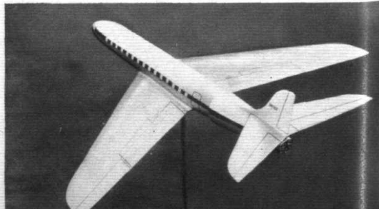
Model of the A.W.167 transport project, with five tail-mounted Sapphires.
