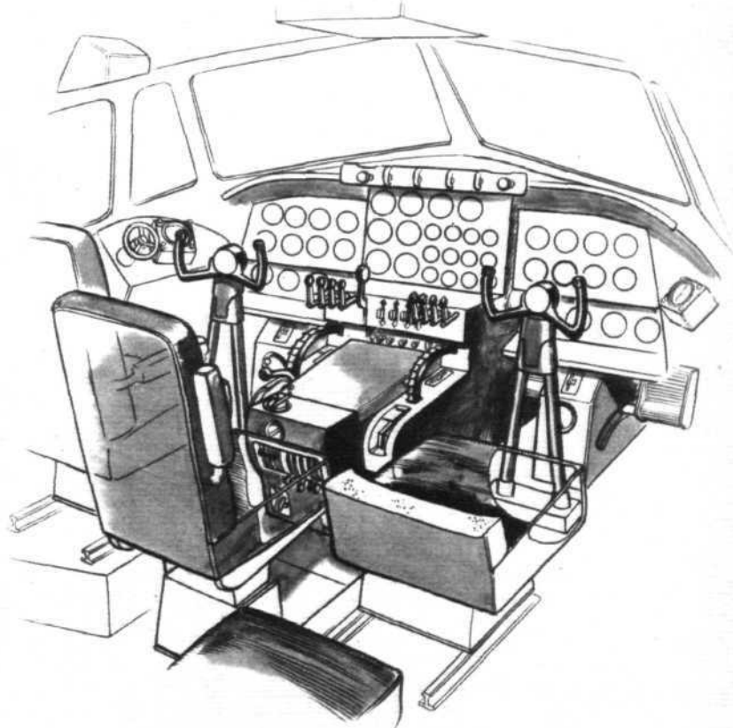
The Electra cockpit is designed to S.A.E. recommendations and provides for a flight crew of two or three, with a fourth seat (visible in the foreground) for a supernumerary. On the pedestal are radio controls and, to port, the flight-idle gate release, and flap controls to the rear of the big trim wheels. The fuel panel is on the rear face of this pedestal. Power levers are on each side, sandwiching the four condition levers and the large undercarriage lever. On each side of the fascia is a P.P.I. display for storm-warning radar and the nosewheel-steering wheel is just behind the captain's radar display to port.
