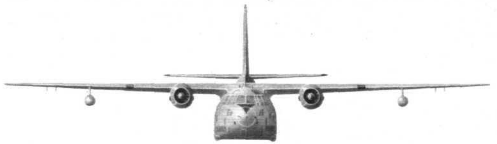
FAIRCHILD C-123B PROVIDER (Two Pratt and Whitney R-2800-99W) Span ... .. 110ft Length ... .. 75ft 9in
