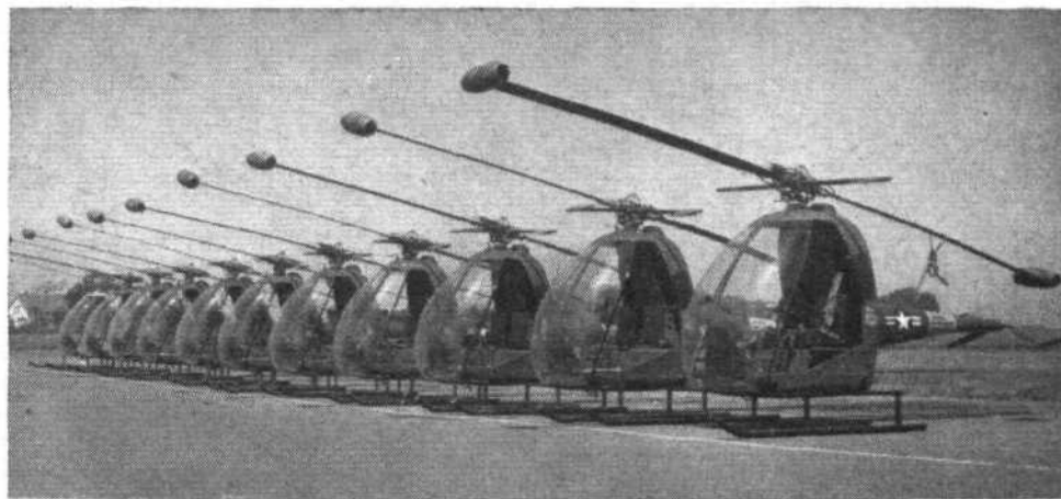
HORNETS: Hiller H-32 ramjet helicopters (the type is popularly known as the Hornet) before delivery to the U.S. Army from Palo Alto, California. Field evaluation will be undertaken at Fort Rucker, Alabama. Glass-fibre is used extensively in the construction of these tiny two-seaters.
