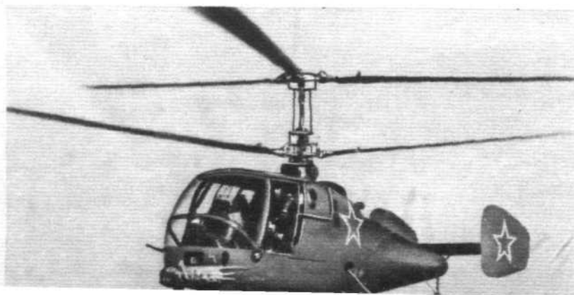
Smaller than it looks in this view, the Kamov Ka-15 is in production for the Soviet Air Force as a general-purpose machine.
