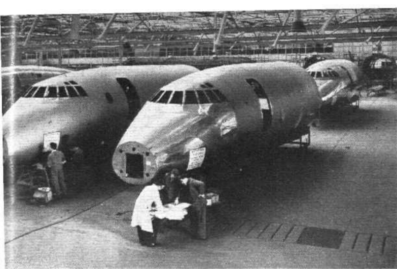
Nose sections of B.O.A.C.'s Britannia 310s coming out of the jigs.
