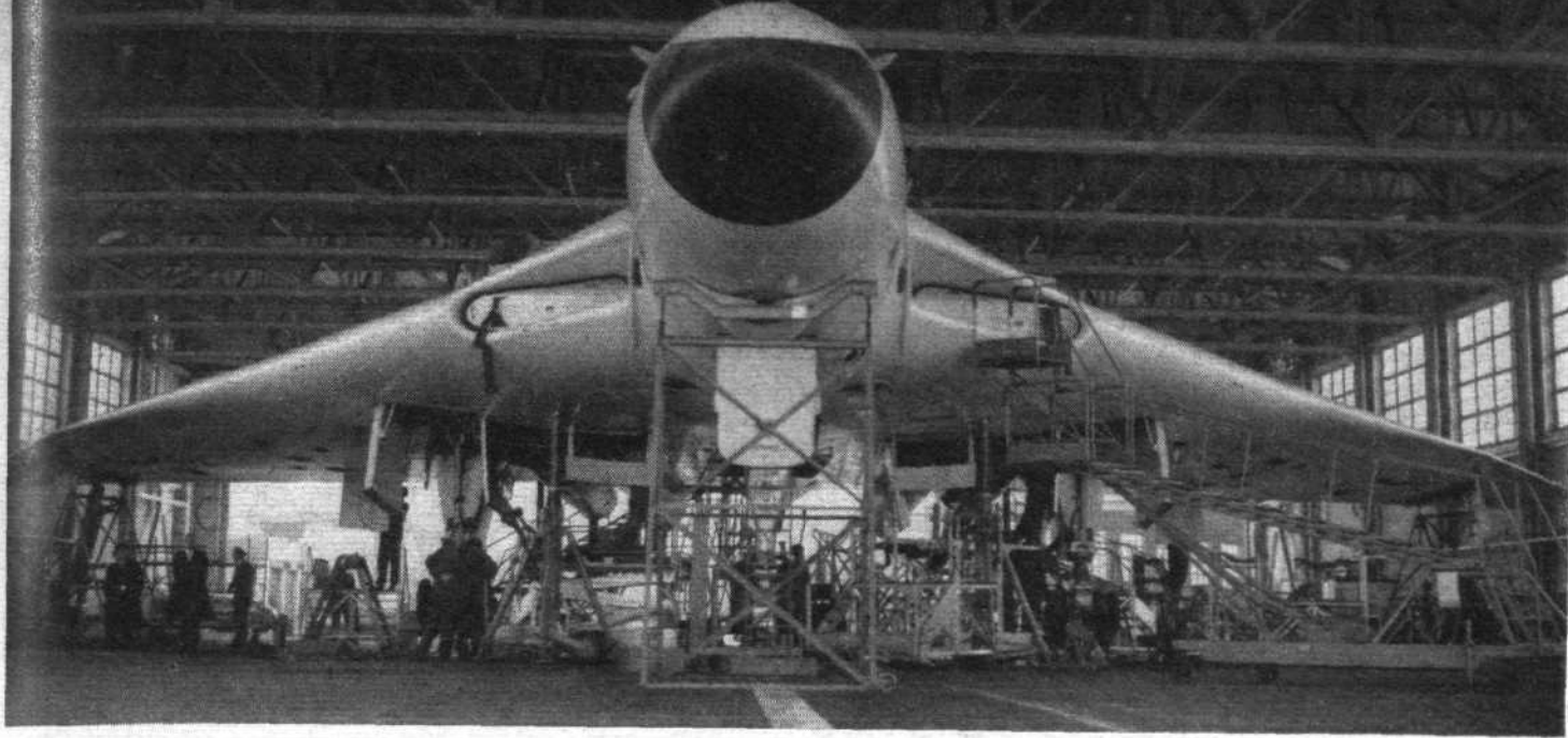
A Vulcan B.1 undergoing a minor inspection at Waddington. Most servicing operations are performed from beneath the aircraft.
