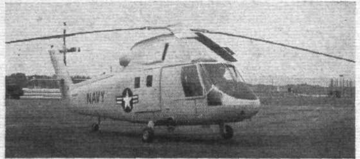
WINNER of a U.S. Navy Bureau of Aeronautics design competition for a utility helicopter is the Kaman HU2K, powered with a General Electric T38 turbine, and shown as a mock-up.
