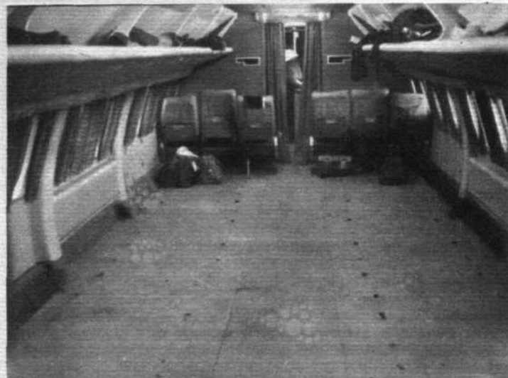
For the record flight to Tel-Aviv 11 rows of tourist seats were removed, as shown here, because full pressure-refuelled tankage could not be obtained at New York.
