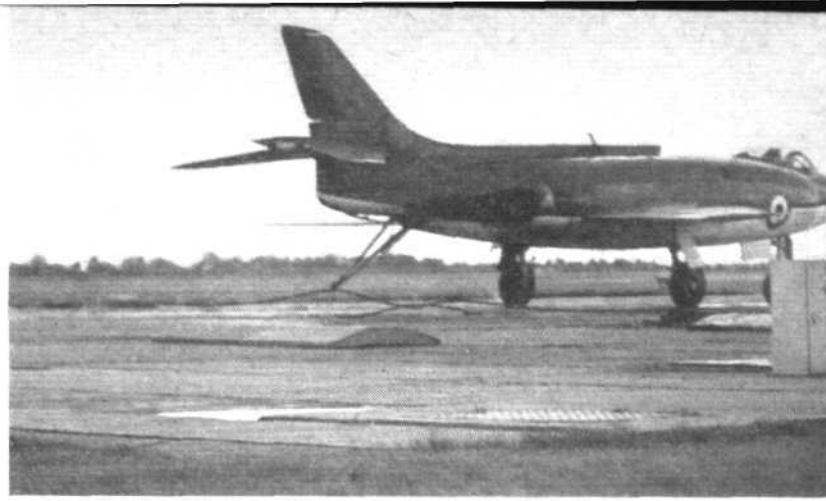
Arrest of a Vickers-Supermarine Scimitar during RAE trials
