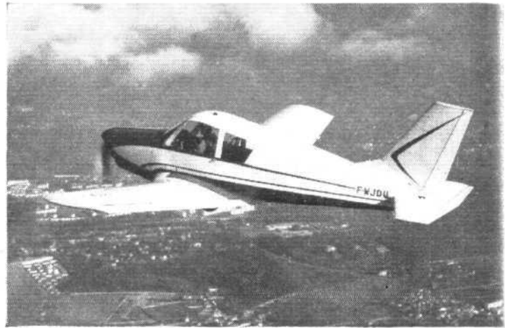
Very like the Piper Comanche, but smaller and only half as expensive, the new French GY80, described in col 1, cruises at 156 m.p.h. with four occupants, full fuel and baggage. Production begins this summer
