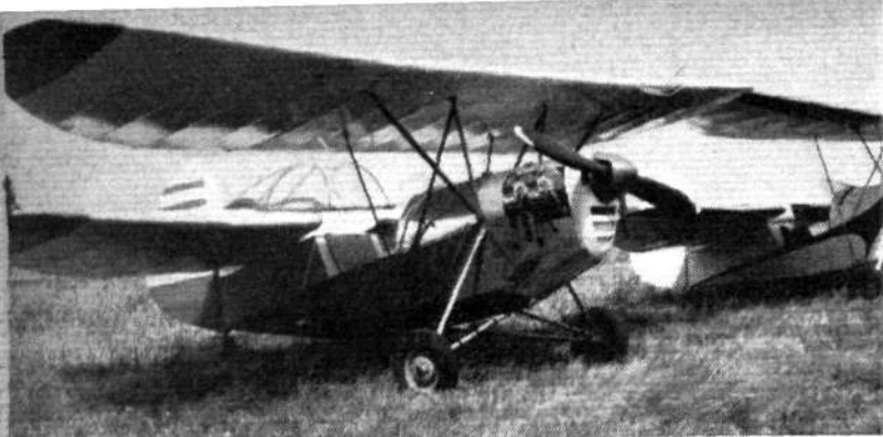
The HM.360—latest single-seater Flying Flea available to amateur constructors—referred to by Mr Best-Devereux
