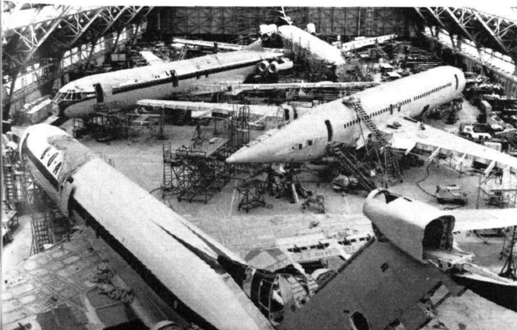
The unpainted VC10 to the right of this picture is the first of 30 Super VC10s for BOAC. Now in one of the two final assembly hangars at Weybridge, this aircraft now has its wings attached. A note on VC10 progress appears on this page
