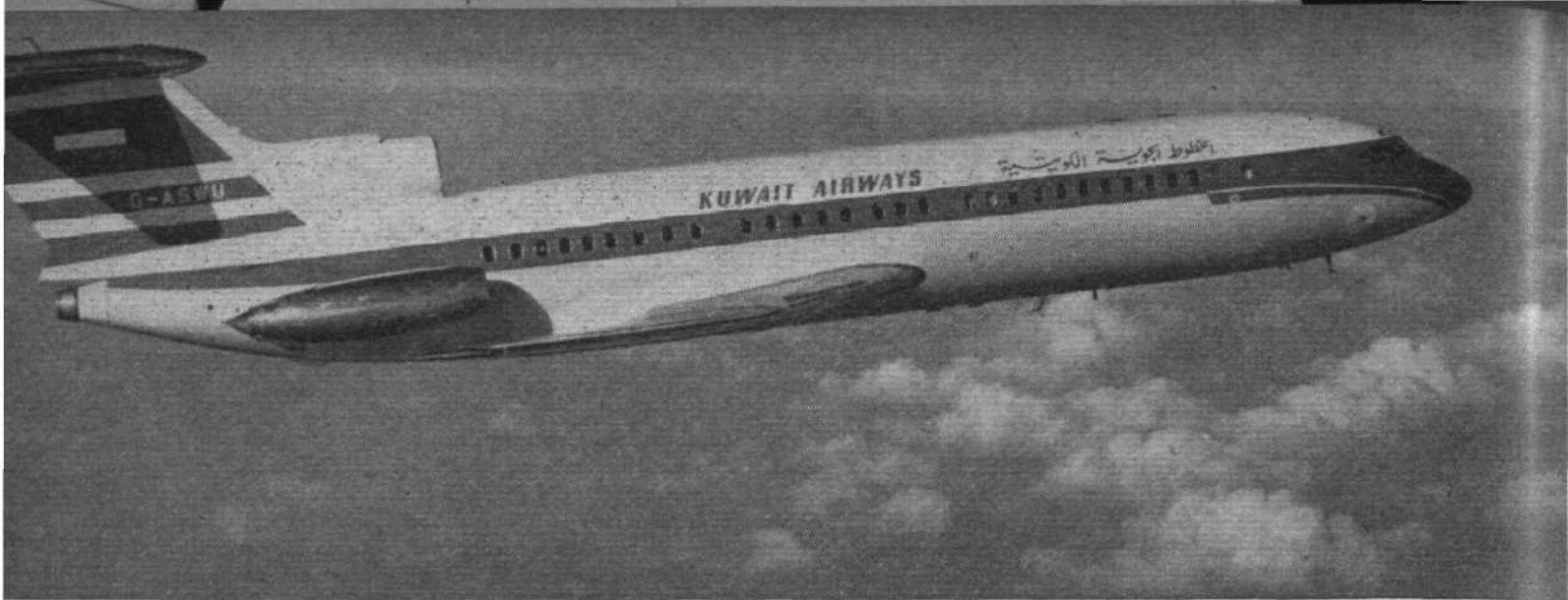
The first of two Trident 1Es (three Rolls-Royce Spey 25 turbofans) ordered by Kuwait Airways was airborne for three hours on its maiden flight on November 2. It was a first flight, too, for the more powerful Spey 25—a type also destined for later marks of the BAC One-Eleven
