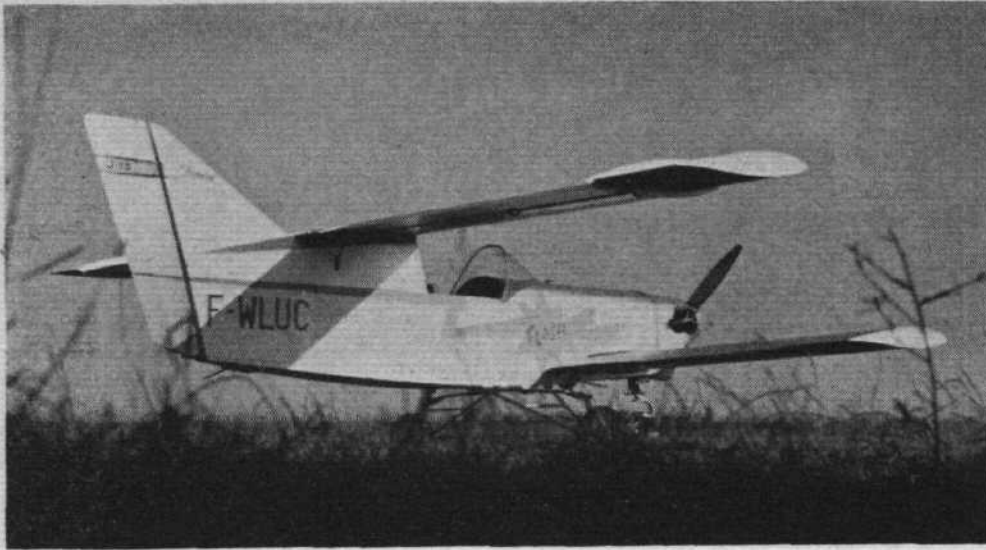
Super Staggered This home-built monoplane (biplane?), designed and constructed by Jo Desprez, of Morlaix in Brittany, is reported to "incorporate novel devices for low-speed control"
