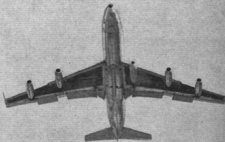
The attachment or removal of El Al's engine-carrying "fifth pod" on the 707-420s takes only 32 minutes
