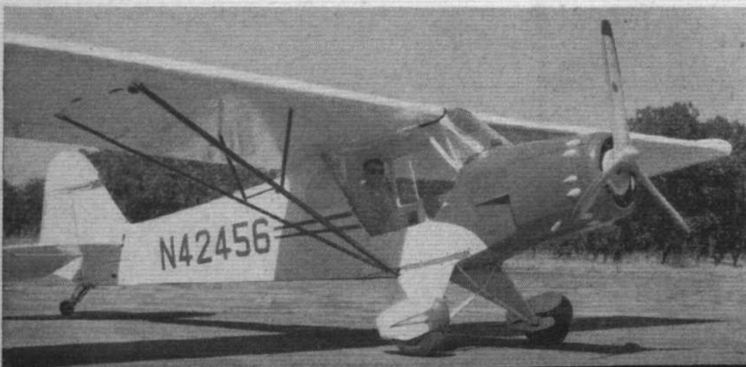
Mr Ole Fahlin, once the manufacturer of Fahlin propellers and now an engineer with Lockheed Missiles, has re-engined this 1945 Piper J-3 Cub with a famous British engine of the inter-war years—the 85 h.p. Pobjoy R geared radial
