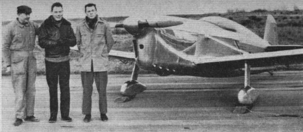
The French René Leduc RL.21 (147 h.p. SNECMA Régnier 4L.00) recently established two class C1a world records for aircraft of under 500kg gross weight. The RL.21, which already held five other world speed records in the C1a and b categories, averaged 217 m.p.h. over a 100km closed circuit and 208 m.p.h. over a 500km course. Left to right: M Prosper, chief mechanic; M Leduc, designer and constructor; and M Raymond Davy, pilot
