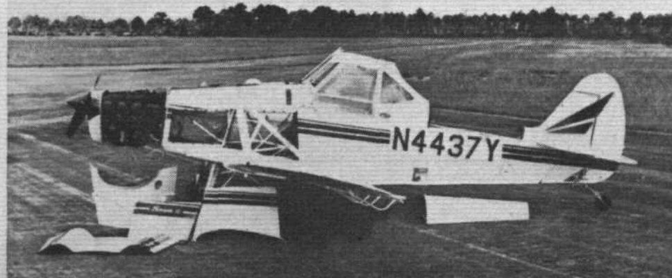
Piper's improved Pawnee C is rapidly adaptable for carrying and delivering either 150gal of liquids or 1,200lb of solids. Improvements include removable top decking, better cockpit ventilation and a "pressurised" fuselage to keep out chemicals
