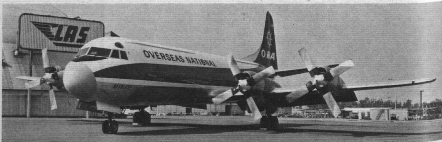
Conversion of 34 Electras to all-cargo and combination/convertible configurations for four airlines by the Lockheed Aircraft Service Co is in progress. Below is the first completed all-cargo (windowless) conversion for Overseas National; note the strengthening strake above the closed door. Above is the upward-sliding plug-type windowed door for a convertible variant. See story on this page
