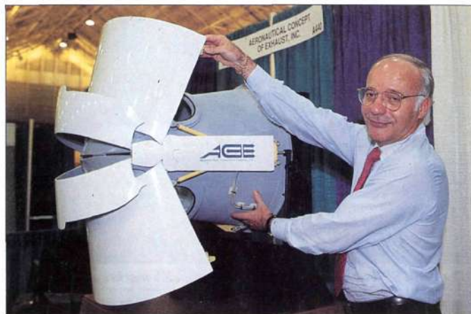
New thrust reverser/variable nozzle design increases efficiency, claims Lair
