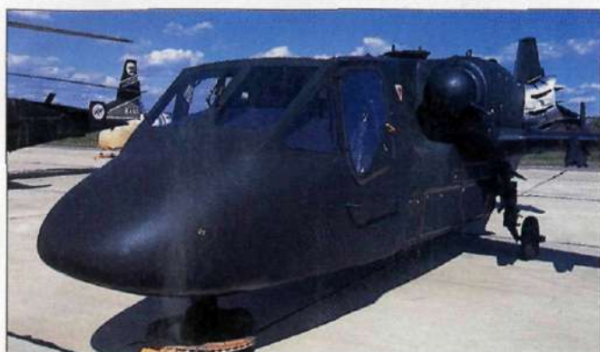
Kamov's two-seat Ka-52 is a derivative of the Ka-50, but has a modified cabin
