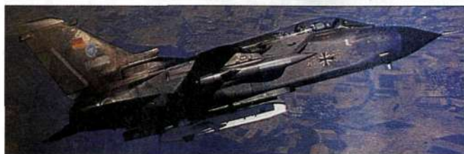
Stand-off over Germany as Tornado conducts captive fire trials with KEPD350
