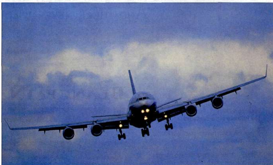
The Il-96M prototype is still the only flying example of the PW2000-powered model
