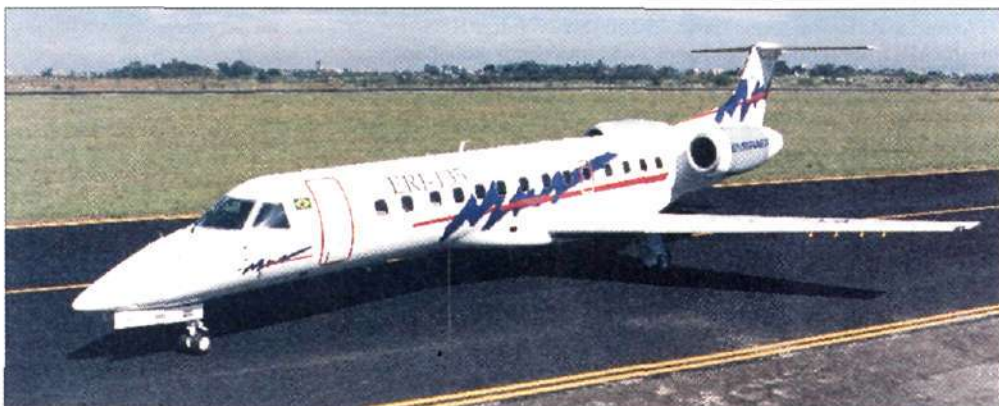
The latest Embraer regional jet, the 37-seat ERJ-135, has been rolled out and could be joined by larger models
