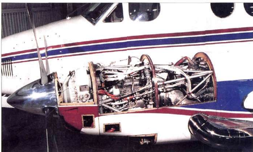
Re-engineing the Beech King Air B100 with the -10 requires new propellers and other changes
